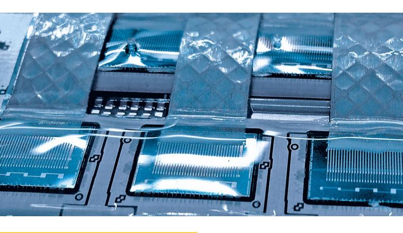
Light-curing adhesives are primarily used in connection technology where rapid curing is required. These one-component products cure at room temperature within seconds after irradiation with UV light. This allows very short cycle times, even with large numbers of pieces.
