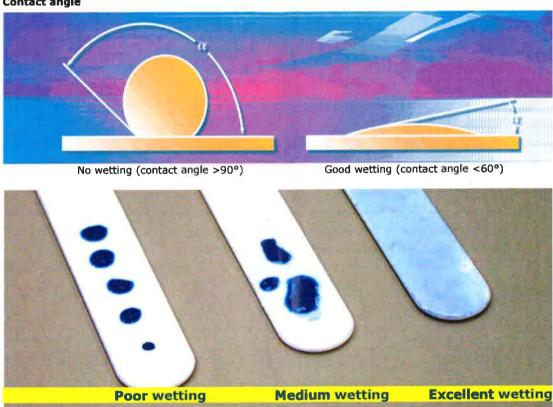
If the wetting of the polymer is insufficient, a surface pre-treatment (mechanical, chemical or physical) is inevitable.
